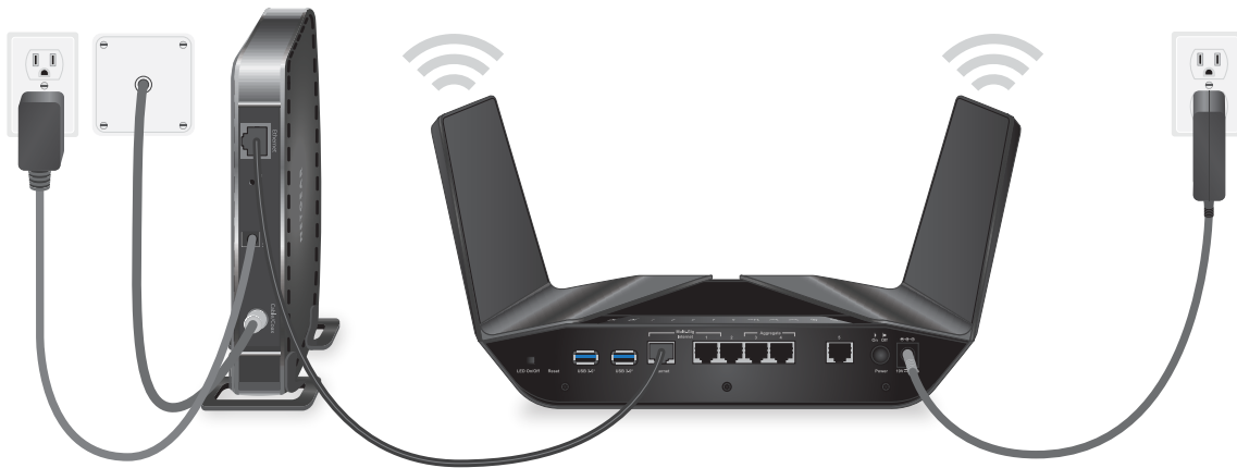
Figure 6. Cable your router
