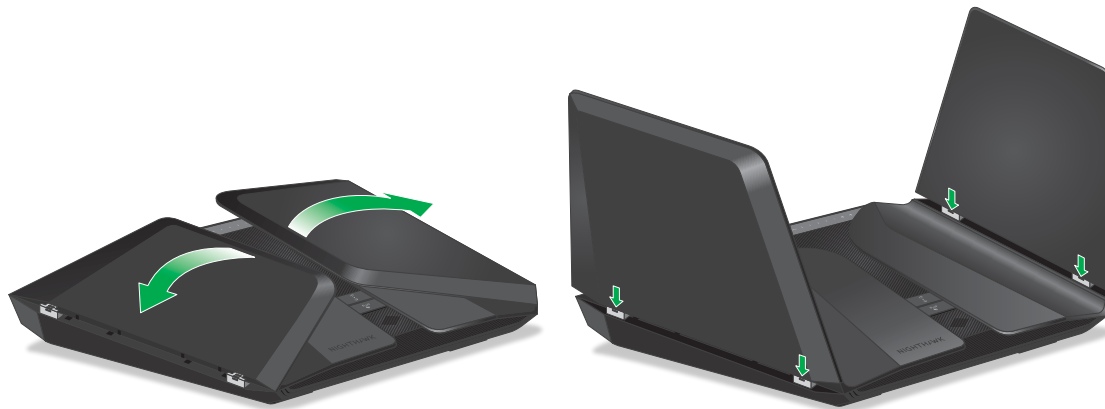
Figure 4. Position the antennas
