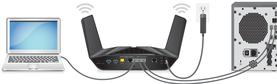
Figure 7. Ethernet port aggregation
