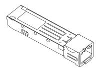
The AXM765 SFP+ module is a low-power, high-performance, multi-gigabit 10G/1000BASE-T transceiver. The AXM765 delivers 10 Gb network connectivity with cabling up to 98.5 feet (30 meters) and delivers 1G network connectivity speed through 328 feet (100 meters) of Category 5e (Cat 5e) or Cat 6 Ethernet cable.
