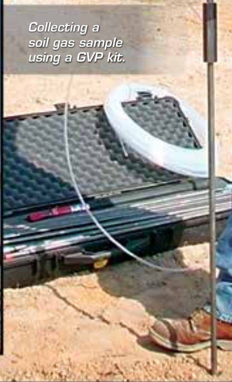
Soil gas sample being collected using a 3' GVP rod with a regular 5/8" threaded slide hammer.
