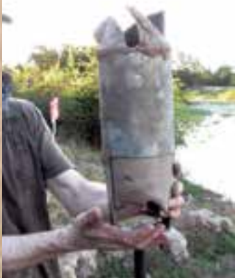
5" diameter regular soil and mud augers utilize three cutting teeth rather than two.
