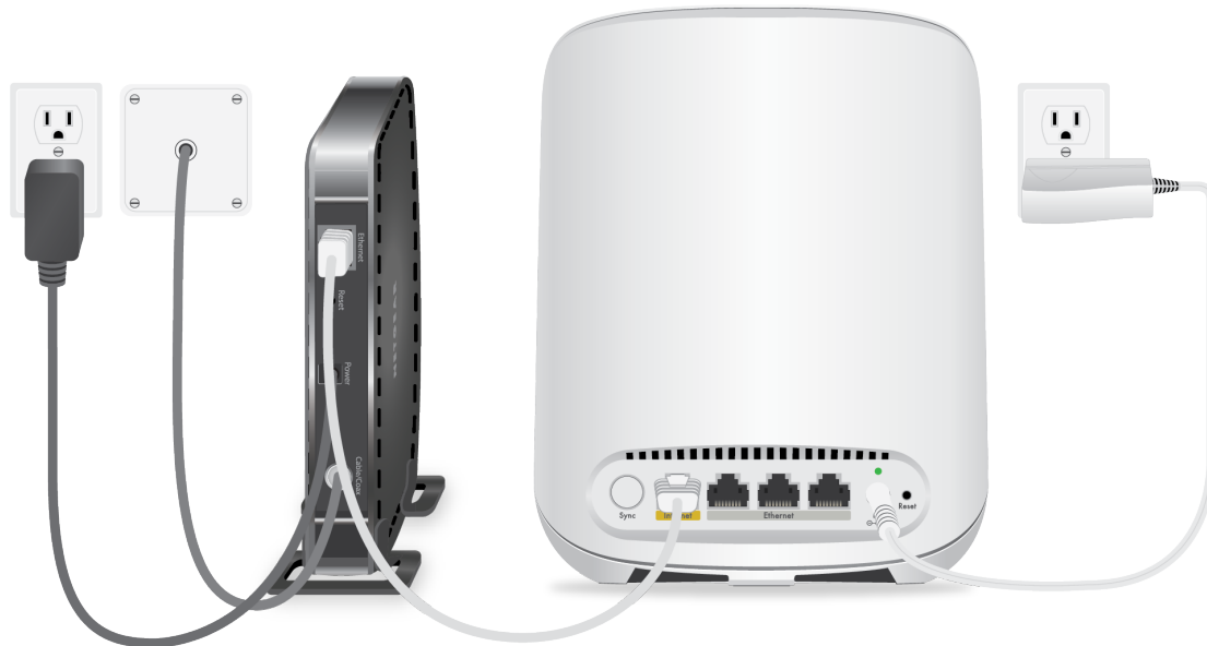
Figure 3. Connect the router
