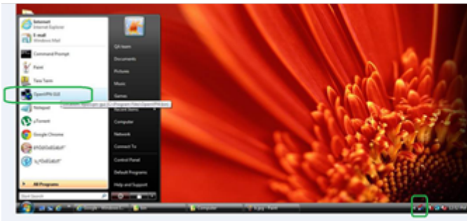
Figure 5. The OpenVPN icon displays in the Windows taskbar.
