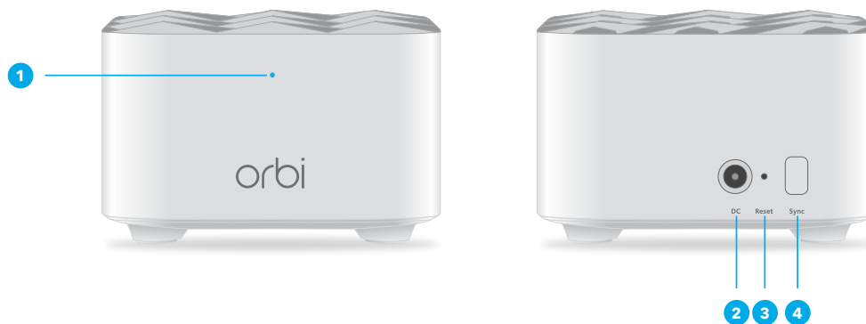
Figure 2. Orbi satellite front and back views
