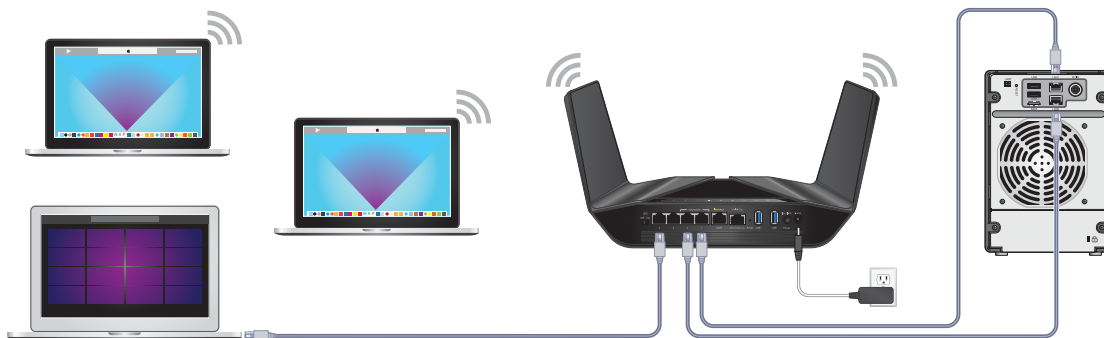
Figure 7. Ethernet port aggregation to a LAN device
