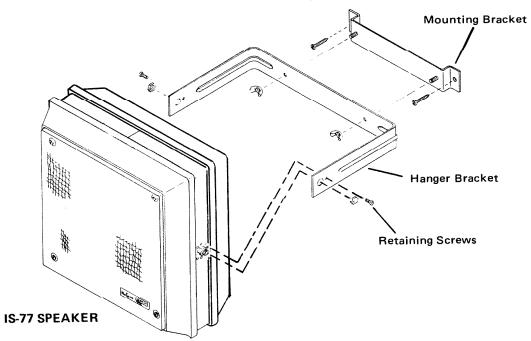
For use with IC-21, ICA-31 and ICA-41 Remote Controls in IA-19 Weather Shield and 2515 Stereo Outside Remote Control.
