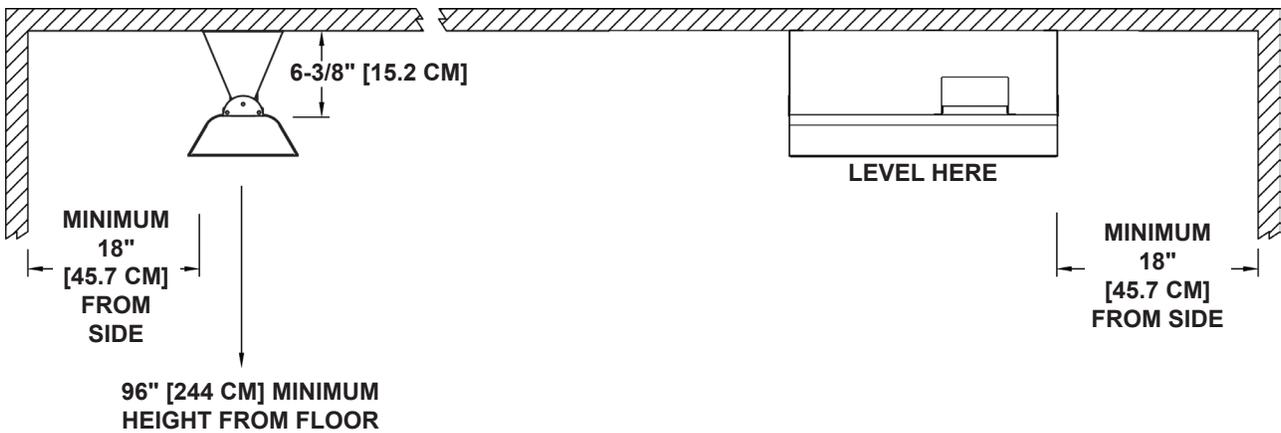
Heater must be installed with the Quartz horizontally level. For maximum tube life, use a carpenter's level tool to find the optimum level position for the heater's body. Always maintain the minimum clearances from the heater body to any combustible materials.
