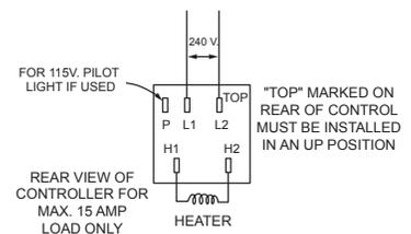
Connect power with flexible conduit or appropriate cord to allow heater to be swiveled.
