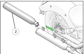
4. Loosely install retained bolts ©, washers ® and exhaust isolators ® into recess in exhaust mount and loosely install bolt © to secure lower muffler to exhaust mount.
