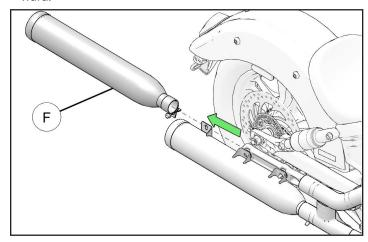
6. Remove lower muffler (a) by gently moving muffler up and down and side to side while sliding muffler assembly rearward.
