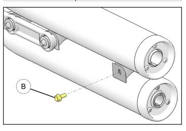
6. Make sure mufflers are properly aligned, torque bolts (B) and (C) Then torque nuts (A) on muffler clamps. Ensure clamp orientation is correct.
