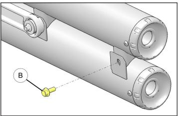
4. Remove two bolts (a) washers (b) (if installed) and exhaust isolators (b) (if installed) connecting upper muffler to exhaust mount.
