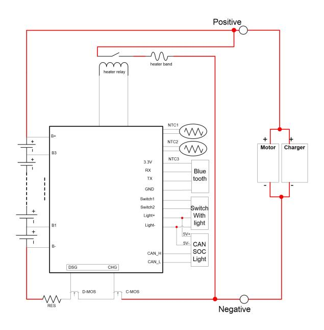
Figure 1. Schematic Diagram of Battery System
