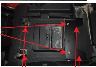
3. You can now slide your seat into the bracket and bolt down the front using part A
