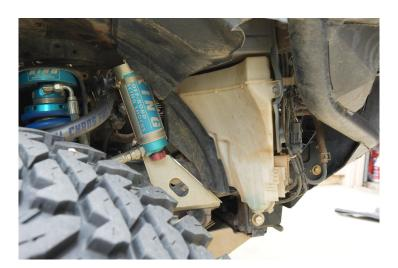
3. Remove the three 10mm bolts holding the factory reservoir in. Each bolt location is shown circled in RED in the next three images.
