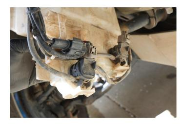
6. After removing the pump gaskets, clean off and reinstall the two gaskets on your new washer fluid reservoir.
