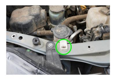
2. Uncover factory reservoir by removing liner until it is fully exposed as shown below.
