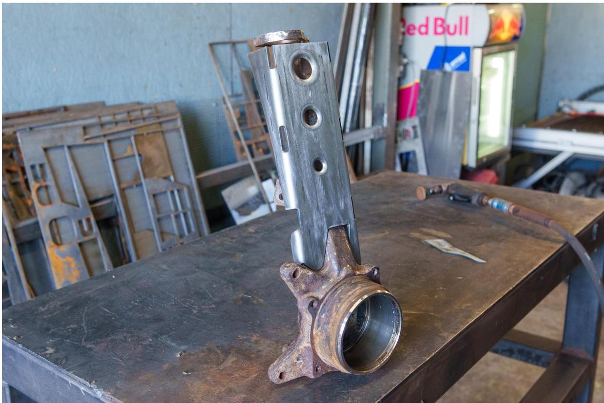
4. Place the TOP PLATE at the top of the MAIN GUSSET (shown below). Once fitment is verified, tack the TOP PLATE to the MAIN GUSSET. Do not yet tack it to the spindle.
