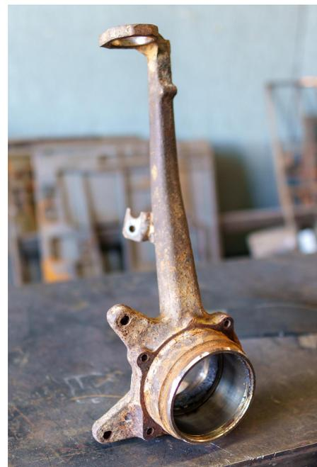
2. Place the gusset pieces on the spindle temporarily and mark areas that need to be cleaned. Refer to photos in the next steps if you are unsure of where to place the gusset parts. Remove gusset parts and remove surface rust, paint and grease from the spindle with any type of sander and degreaser in the areas that will be welded.
