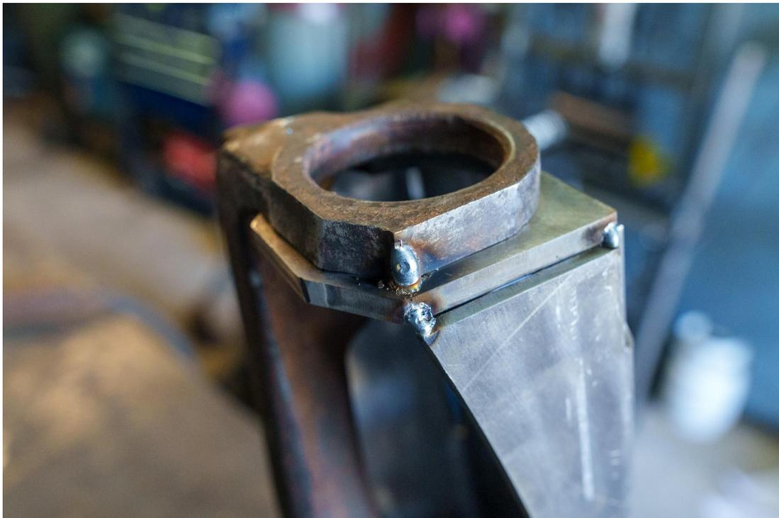
6. Remove the upper ball joint or uniball adapter. These parts should not be subjected to the heat from welding.
