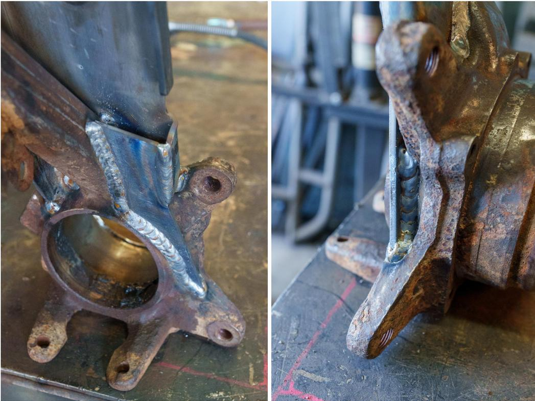
**10. Wait for the spindle to cool. Do not try to cool it with water. Once it is fully cool, paint the spindle with spray paint to prevent rust. Do not weld inside the upper ball joint hole or inside the wheel bearing area. Cover any bolt holes to prevent paint from getting into the threads.**
