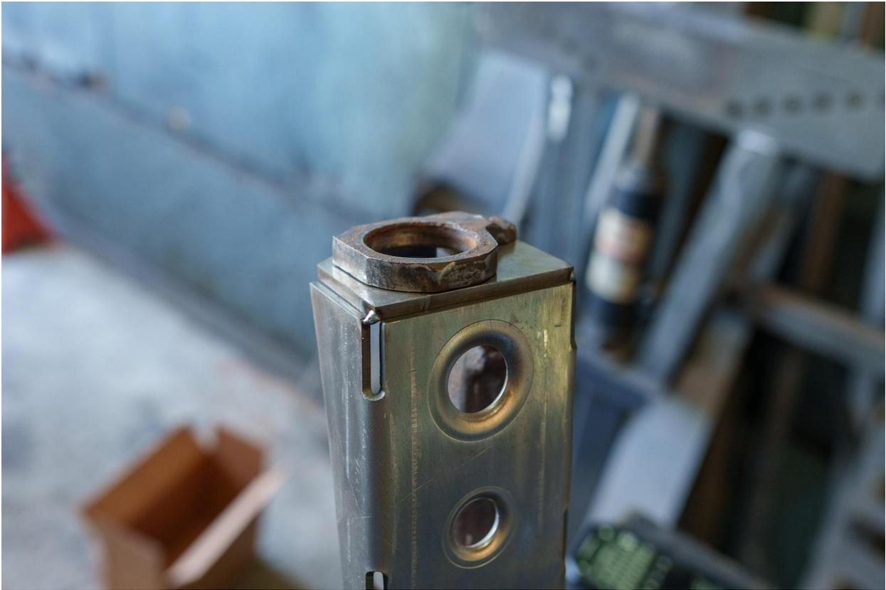
5. Now that these two parts are tacked together, align them so that the hole of the TOP PLATE is centered as perfectly as you can with the upper ball joint hole. Make sure that the hole of the TOP PLATE fits around your upper ball joint or uniball adapter. The spindle in the picture example below did not have an adapter in the spindle hole but usually you would want to still have it installed to verify fitment. Tack the gusset to the spindle so it does not move.
