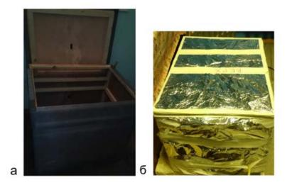
Fig. 1. A Faraday cage covered in (a) a metal mesh, (b) a metal mesh and aluminum foil.
