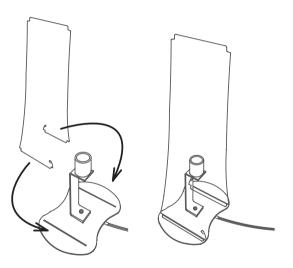
While pressing the lower part of the harp from the side, insert it into the groove of the base plate.
