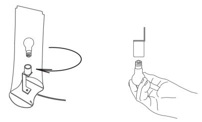
Place the light bulb into the socket and screw it in firmly.
