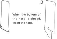
If the bottom of the harp is open, cross the harp and bend it to A state, then insert
