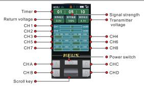
[Power switch]: long press to turn on and off, short press to return.
