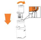
Attach the feeding cup and rotate it clockwise.
