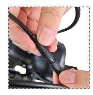
Connect the LCD display joint to the controller.
