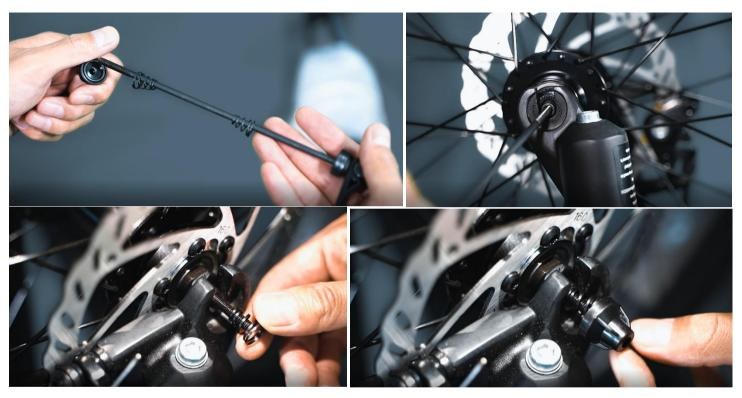
• Remove the thumb nuts and one of the cone springs, insert the quick release skewer through the hub.
