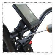
Put LCD display in the middle of the handlebar, then use 3mm hexagon to fix the screws.
