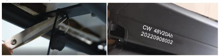
Find the keys located under the saddle and remove them. Use the key to unlock the battery. Remove the battery to avoid possible damage during installation.
