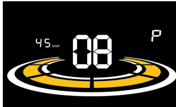
Figure 6-8 Speed limit setting interface
