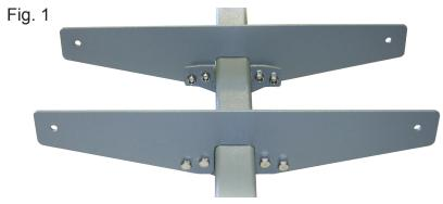
**Step 2.** Place the motorcycle rack between the support brackets, noting the ramp mounting holes on the rack are on the side where you will be storing the ramp. Install the four M8x40 bolts (E), washers (G), and nuts (H). Securely tighten all
