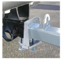
**Step 4.** The ramp (B) stores on the motorcycle rack with the two supplied bolt, nut, and wing nut assemblies (K).
