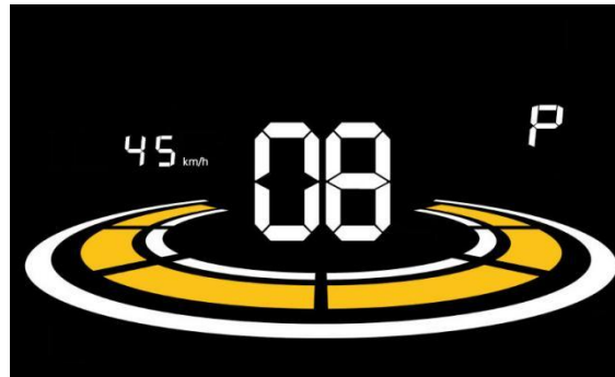
Figure 6-8 Speed limit setting interface
