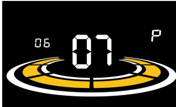
Figure 6-7 Number of speed sensor magnets setting interface
