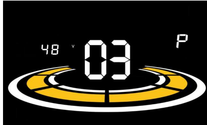
Figure 6-3 Rated voltage setting interface
