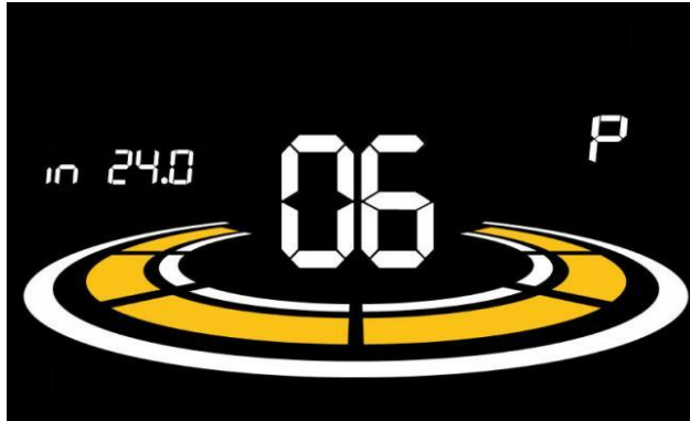
Figure 6-6 Wheel diameter setting interface
