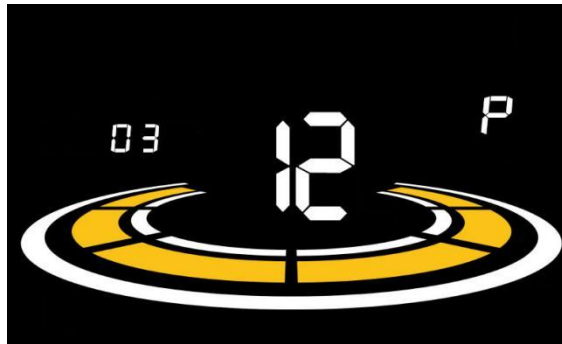
Figure 6-12 Pedal assist Start-up intensity setting interface
