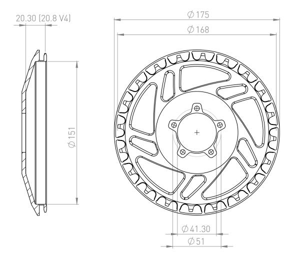
Note the package includes a 2mm Spacer so that you can space the Bling Ring out to the same offset as the original Bling Ring offset. We decided to offset the Bling Ring an extra 2mm so that useres could try get that perfect chainline for the 73mm BB frames. If you are building a 73mm BB frame try installing without the spacer. You should have at least 1.5mm gap between the ring and chain-stay.
