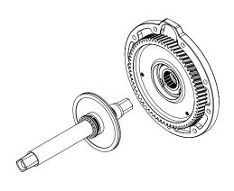
**3. Slide the remaining axle assembly in.** Note: Grease all touching surfaces to make maintanance easy.
