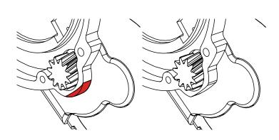
3. Using a file, carefully remove highlighted material to the scribbed line making it the same shape as the Lekkie Drive Cover HD. You may also need to trim the paper gasket. Note: We advise covering the pinion and inside of the motor so that the metal filings do not make it into the motor.
