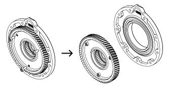
4. Screw 3 M4 screws into the back side of the drive gear until they are touching the bearing. Start turning one screw one turn, then the next screw once, then turn the next screw one turn, then the next. Repeat until the gear is removed.
