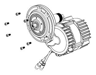
4. Install paper gasket then slide the new drive assembly in. Clean, apply Loctite 243 to threads, and install the six M5 drive cover bolts. Tighten to 6Nm.
