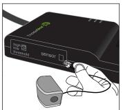
Plug the multi-sensor into the port on the side of the powerstrip that looks like a phone jack. Adjusts the thresholds level low-15W/high-50W based on TV/control outlet power consumption.
