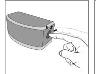
To configure countdown timer: press and hold button for 10 sec. Press 1X for 75 mins, Press 2X for 135 mins, Press 3X for disable the countdown timer buzzer. After countdown timer is set, the LED will flash the number of times that timer has been set to.
