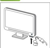
Attach multi-sensor to your TV in the location determined in step 5. The ideal sensing range is 6 to 12 foot away from the TV.
