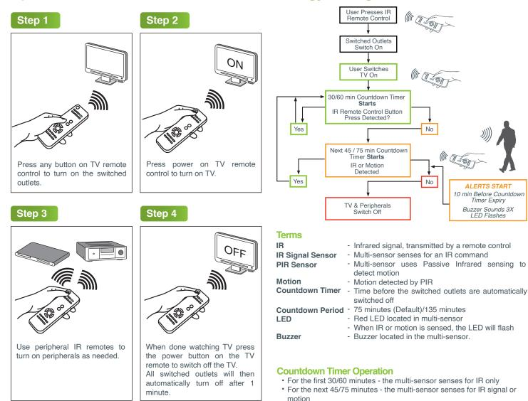
After 75 minutes/135 minutes - the switched outlets will switch off automatically if no IR or motion has been sensed.
