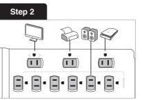
Plug peripheral electronics into the outlets on the powerstrip labeled "switched."
