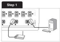
Plug in devices that require continuous power into the always-on outlets (e.g., modem, CPU).
