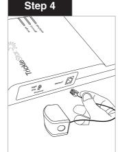
Plug the SensorClick motion sensor into the port on the side of the power strip that looks like a phone jack and is marked "sensor".
