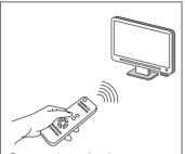
Press any button but the power button on any Infrared (IR) remote control to turn on the switched outlets. You may hear a click as power is supplied to the switched outlets. The green "switched" LED on the top of the power strip will illuminate.
