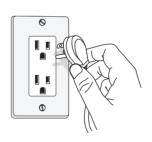
Plug the power strip into a grounded outlet. The ground and surge lights on the power strip will illuminate, indicating that the power strip is properly grounded and surge protection is active.
