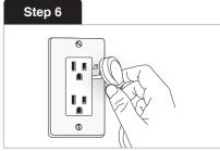
Plug the powerstrip into a grounded outlet receptacle. The ground and surge lights on the powerstrip will illuminate indicating that the powerstrip is properly grounded, and that surge protection is active.
