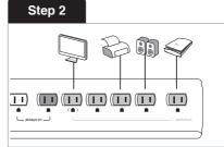
Plug peripheral electronics into the outlets on the powerstrip labeled "switched."
