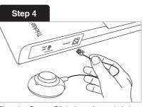
Plug the SensorClick timer footswitch into the port on the side of the power strip that looks like a phone jack and is marked
