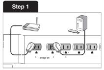
Plug in devices that require continuous power into the always-on outlets (e.g., modem, CPU).
