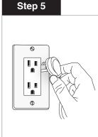
Plug the power strip into a grounded outlet receptacle. The ground and surge lights on the power strip will illuminate indicating the that power strip is properly grounded, and that surge protection is active.
