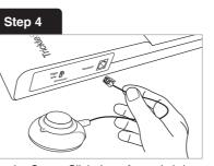
Plug the SensorClick timer footswitch into the port on the side of the power strip that looks like a phone jack and is marked "appear"
