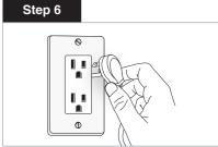
Plug the powerstrip into a grounded outlet receptacle. The ground and surge lights on the powerstrip will illuminate indicating that the powerstrip is properly grounded, and that surge protection is active.
