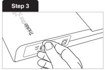
Set the adjustable threshold switch to "low" when using a monitor as the control device and "high" when using the TV as a control device.
