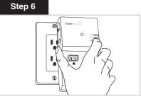
Plug the powertap into a grounded outlet receptacle. The ground and surge lights on the powertap will illuminate indicating that the powertap is properly grounded, and that surge protection is active.
