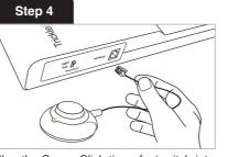
Plug the SensorClick timer footswitch into the port on the side of the power tap that looks like a phone jack and is marked "sensor"
