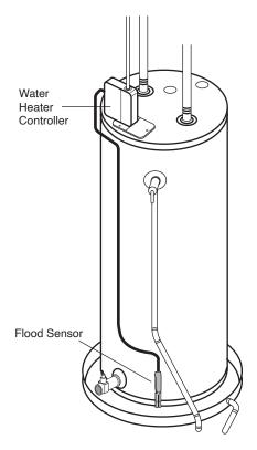
3. Connect the Flood Sensor wire to either terminals of sensor 1 or sensor 2 on your Water Heater Controller.
