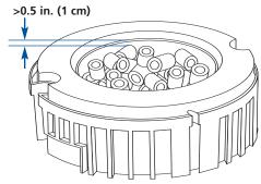
6. Stack the baskets, carefully aligning them, so that all shapes match. Reinsert the T-handles into their vertical slots, and replace the baskets in the filter canister. The foam in the upper basket should be just about even with the top edge of the canister (the output tube, which is affixed to the inside of the canister, will be protruding slightly).
