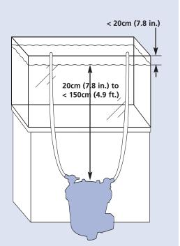
**2.** Place the two rim connectors over the back top edge of the aquarium. Place one just above the spot where you want to place the intake tube; place the other just over the spot where you want to position the output nozzle. Be sure that the long end of the bracket is on the inside of the aquarium.
