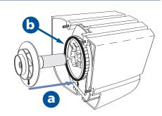
6. Re-attach the pump unit to the canister using the 4 fixing screws with a Phillips screw-driver (cross headed). While reassembling the pump, the 4 fixing screws should be gently screwed until pump motor cover and canister are securely attached. Note: Do not over tighten housing to canister.
