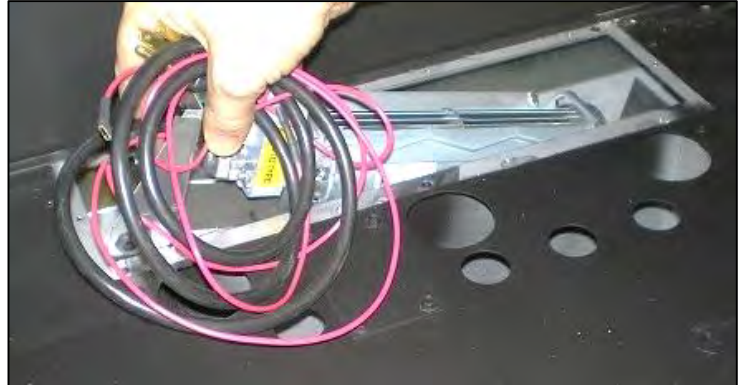
2. Insert Fan Assembly through opening.
