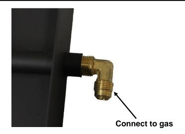
**IMPORTANT:** The minimum inlet supply pressure for the purpose of input adjustment is 5.0 inches (natural gas)in water column. The maximum inlet supply pressure is 10.5 inches (natural gas) in water column.
