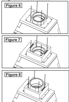
5. If an offset is required after a short run of straight flue, start with a standard 8" high inner flue (MCL-814). The offset will require that the inner and outer flue is flush at the beginning of the offset sections. After the offset is complete, resume the straight stack with a short 4" high inner flue (MCL-414) and continue with 8" high inner and outer sections (MCL-814, MCS-814). At the point
