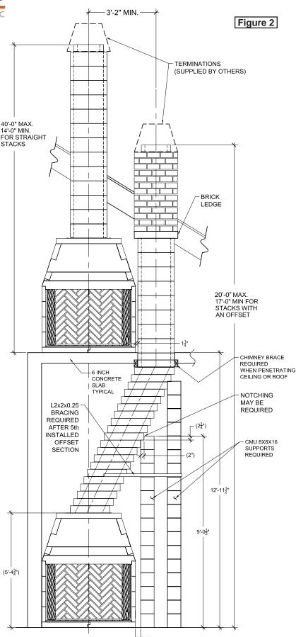
The MCLS-814 Masonry Chimney System consists of the
