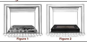
Place Opalescence burner in your fireplace centering the base front to back and side to side. Centering the base allows the case to easily slide over the top of the base. (Figure 1)
