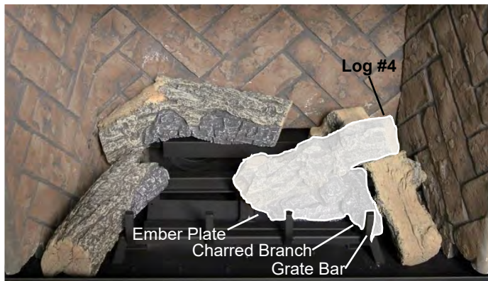
Step 4: Place Flattened Area of Log #4 onto the Ember Plate, making sure it is completely seated. The charred Branch of Log #4 will rest on the end of the Grate Bar.
