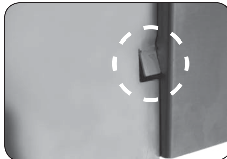
Fig. 22-2 Tab slightly bent in for clearance
