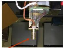
To ensure a tight fit add Teflon Tape to the threads of the heaters bottom connection
