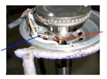
2) The pilot light just flickers but will not stay lit. This tells us that the LPG (propane) in the pilot tube is not sufficient enough to light the pilot and the rate of air is too high. In this case we need to move the pilot tube inward approximately 1/8" to 1/4" to reduce air mixture flow.
