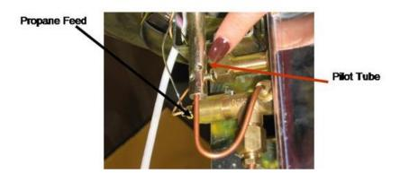
To clean the inside of the pilot tube loosen the holding screw on the side of the pilot tube. Do not unscrew it all the way or it can get lost and the heater will not work correctly. The copper tube that goes into the brass tube is the propane feed.
