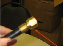
Make sure that the regulator hose has no cracks in it and is sealed around the fitting.
