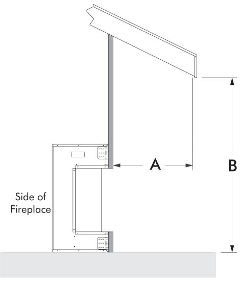
The overhang (A) must extend at least 1/2 the roof-line height (B).
