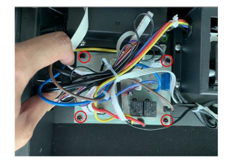
Remove the four (4) screws and unplug to insert a new circuit board
