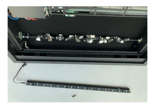
If you cannot remove the wiring out from the slot, loosen the adjustable foot slightly to remove the wiring out from the slot and take the tray light assembly off.
