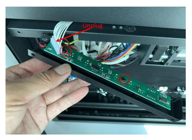
Remove two (2) screws and unplug to replace a new touch panel
