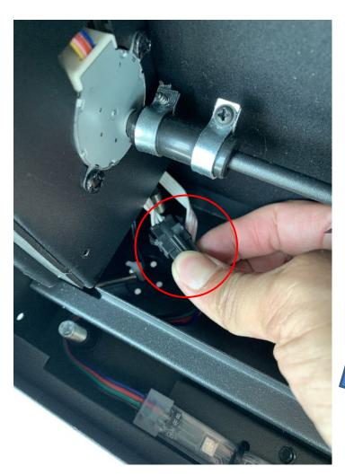
Unplug the tray light from the fireplace and detach the wiring from the slot to take off the tray light assembly.
