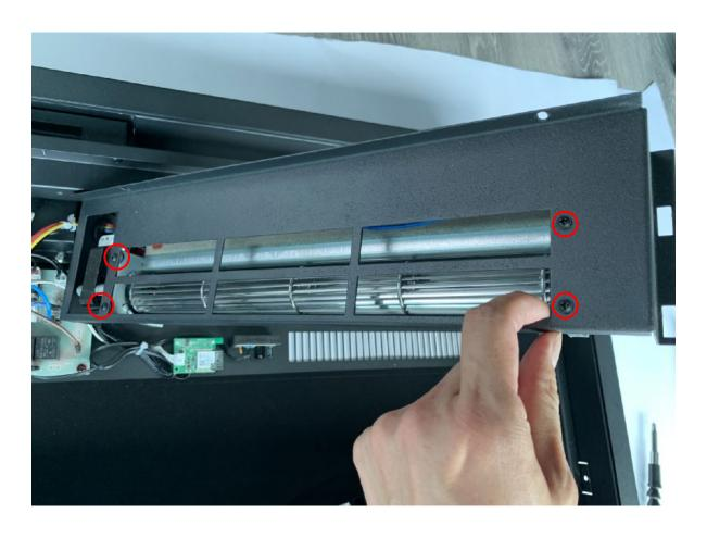
Remove four(4) screws and unplug to replace a new heater.
