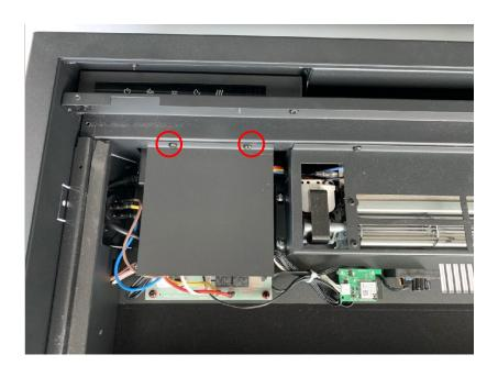
Remove the two (2) screws to take off the circuit board protective panel
