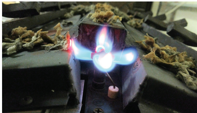
Figure 4.3 IPI Pilot Flame Patterns
