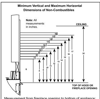
Measurement from fireplace opening to bottom of appliance: 33-9/16". Measurement is taken from the top of the opening, NOT the top of the fireplace.
