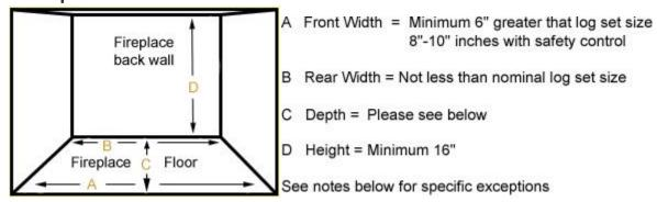
Sizing a gas log set is fairly straight forward and most fireplaces can be sized using the above general guidelines. Certain fireplace shapes (for example, the steep taper and shallow depth of the Rumford Fireplace) may require additional consideration.
