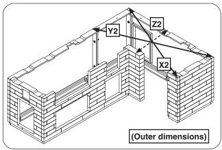
Fig. 14-3 Square unit (then tighten all bolts)
