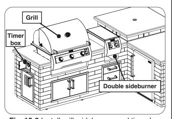
Fig. 18-3 Install grill, sideburner, and timer box
