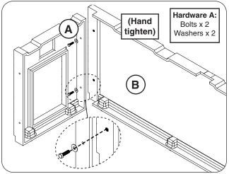
Fig. 11-2 Assemble side wall and rear wall
