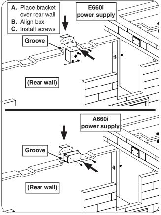
Fig. 17-1 Install power supply box
