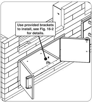
Fig. 16-1 Door/drawer/pantry install detail
