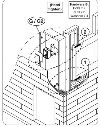
Fig. 13-1 Assemble side wall and outlet box
