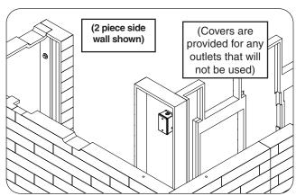
Fig. 13-2 Side wall and outlet box installed
