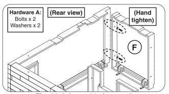
Fig. 12-2 Assemble front wall
