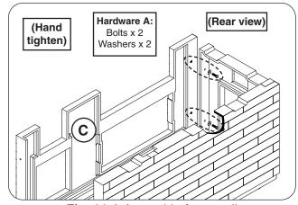
Fig. 11-3 Assemble front wall
