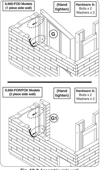
Fig. 12-3 Assemble side wall
