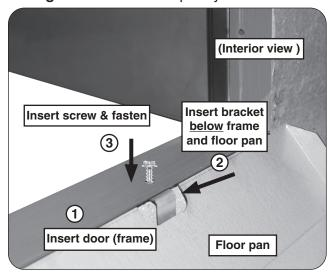
Fig. 16-3 Door/floor pan install detail
