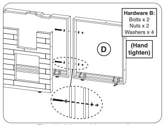
Fig. 11-4 Assemble rear wall
