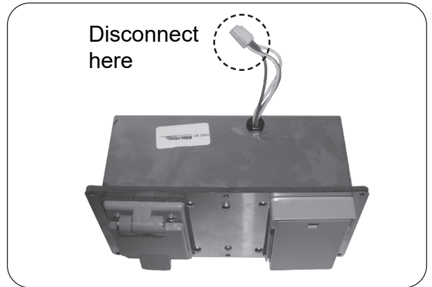
Fig. 41-2 Slightly pull out box and disconnect wire harness
