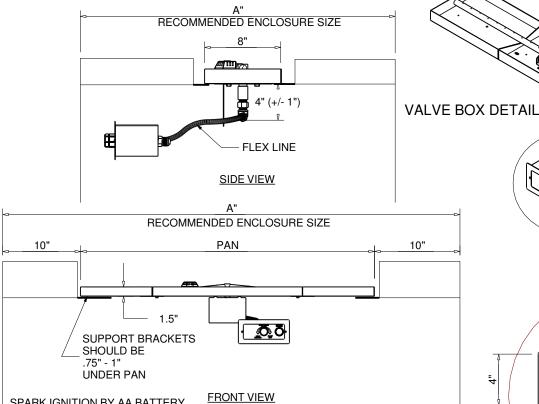
SPARK IGNITION BY AA BATTERY MATERIAL: 304 STAINLESS STEEL
