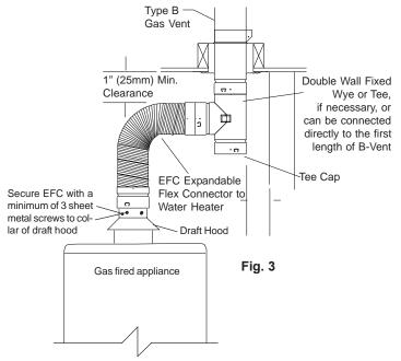
If local codes specify use of a "drip tee", you may incorporate a fixed or adjustable wye or a tee to make the connection to the Type B Gas Vent (see Figure 3).
