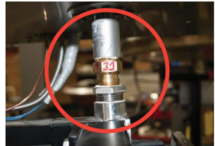
Figure 9.1 – Locating orifice for cleaning
