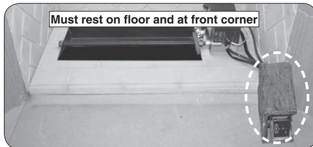
Fig. 10-2 Place heat shield
